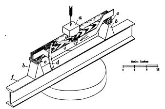
Fig. 4.—Method of testing small beams in bending.
